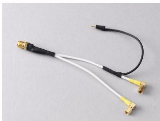
Figure 3-31 **Schematic diagram of the PRB-C adapter cable**
